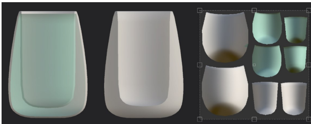
Figure 22. Double-walled thermo glass with and without shell modifier (Neppius 2022)
