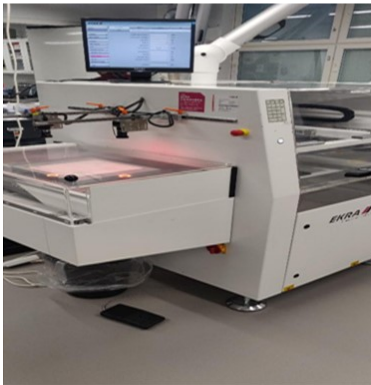
FIGURE 10: Picture showing EKRA E2 screen printer as seen in Print lab Oulu.
