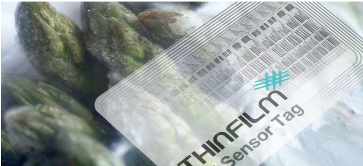
FIGURE 13: Printed thin film sensor tag for product protection (Caliendo 2014)
