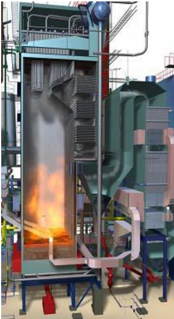
Picture 4. BFB Boiler combustion
