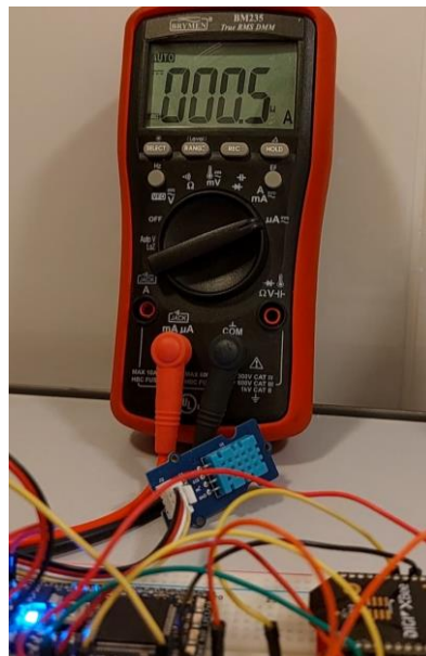
Figure 22. The measured current of R_{shunt} at sleep state
