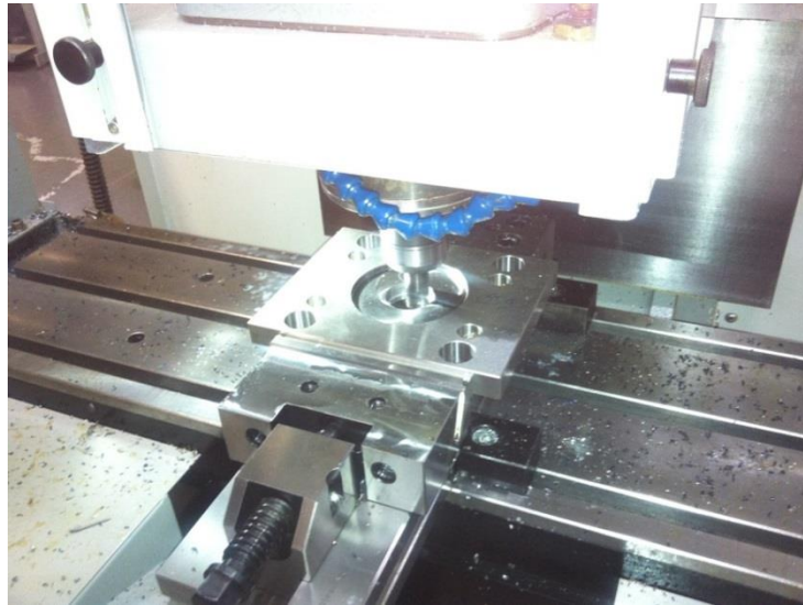
Figure 20. Screenshot of sprue bushing hole drill (CNC drill)
