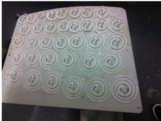
Figure 23. Screenshot of spiral flow test products with varying injection pressure
