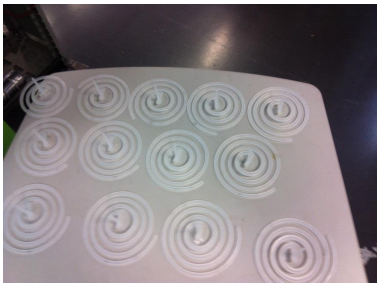
Figure 24. Screenshot of spiral flow test products with varying injection speed
