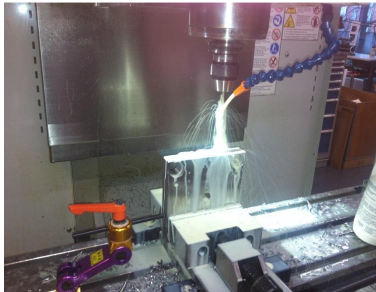
Figure 19. Screenshot of drilling operation performed for cooling channel on mould plates (CNC drill)
