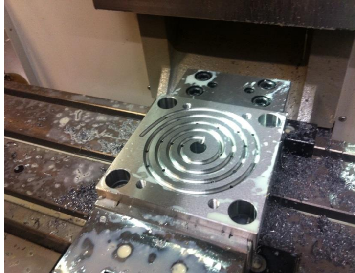
Figure 18. Screenshot of spiral flow test mould cavity manufacturing (CNC mill)
