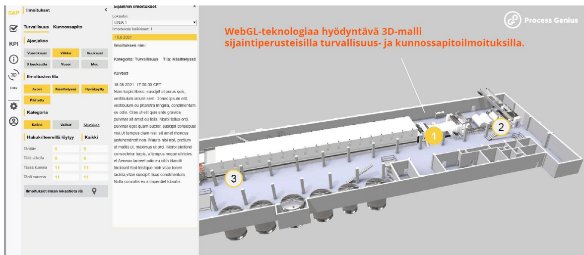
Figure 26 Safety notifications can be placed anywhere on the 3D model (Process Genius, 2021)
