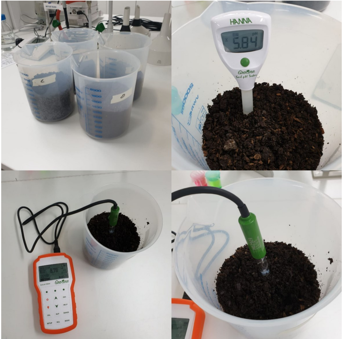
PICTURE 4. Direct soil pH measurement, top right HI981030 and bottom left HI98168 (Author 2021)
