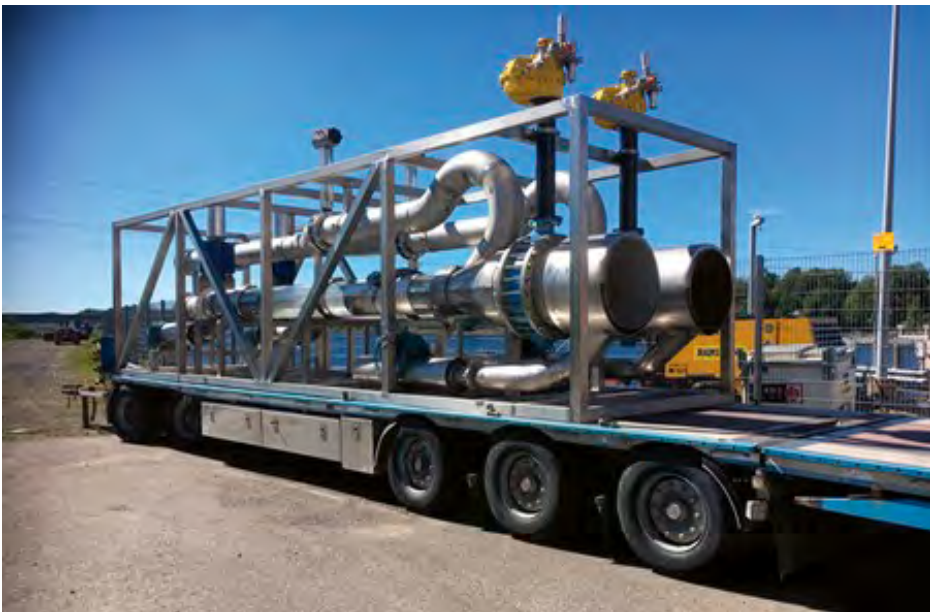
Figure 1. Fishheart – Hydraulic Fishway system.
