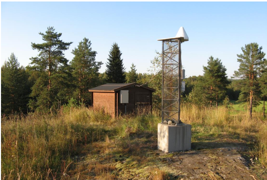
Figure 30. JOEN station showing the antenna mast and the station cottage (Koivula, 2014b)
