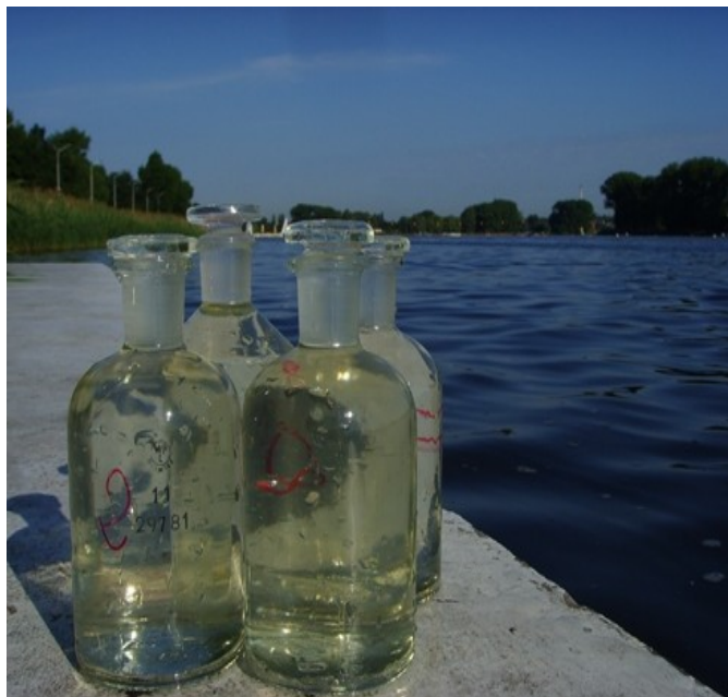
GRAPH 10. Bottles for the collection of samples for analysis of BOD, TOC and dissolved oxygen
