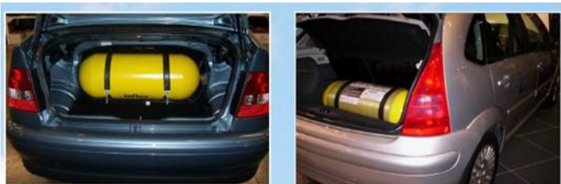
Figure 2: Gas storage tank installed in the trunk of a private car. Source: online-source, NGV market in Latin America.
