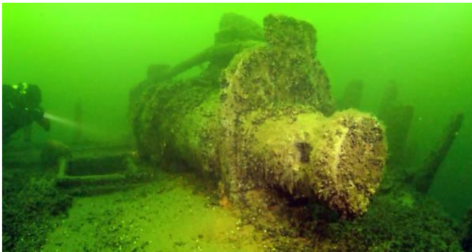
Picture 13. Anchor winch of Osborn & Elisabeth. Pictures are captured from monitoring video, June 2013 © Kari Hyttinen
