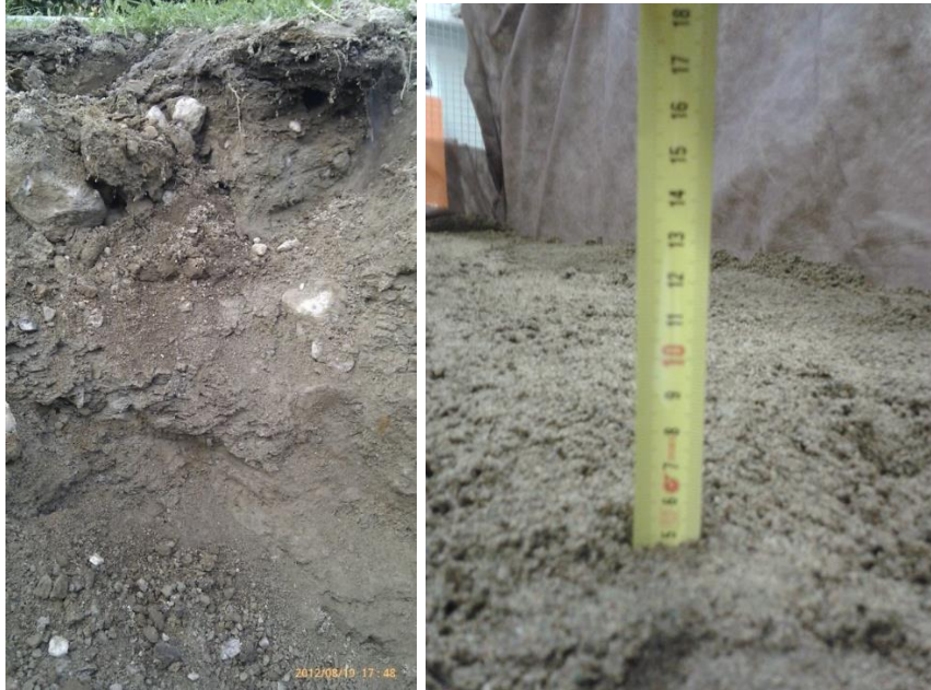
FIGURE 5 Left: Photograph of silty sand from Varpaisjärvi. (Photograph Tuomo Savolainen 2012) Right: Photograph of drying the medium fine sand from Maaninka. (Photograph Paula Kaipio 2012)
