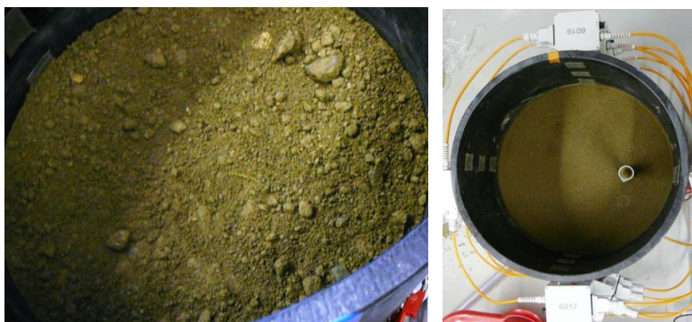
FIGURE 13 Left: Photograph of the bottom layer (silty sand) Right: Photograph of the bottom layer (fine sand) of CASE 3 (Photographs Paula Kaipio 2012)
