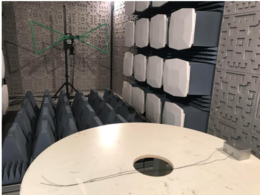
Figure 22. The set-up for Radiated testing in FAC.
