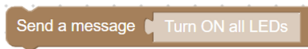
Figure 41. Pall0's "Send a message" block with the value input that contains the "Turn ON all LEDs" block.
