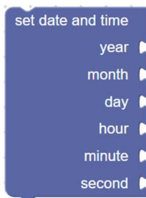
Figure 26. "Set date and time" block from original BIPES project.
