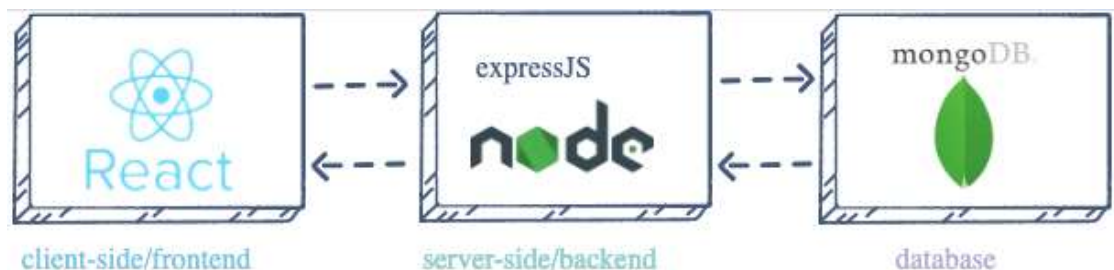
Figure 9. The web portal architecture. Source: MEAN Stack vs MERN Stack 2022.
