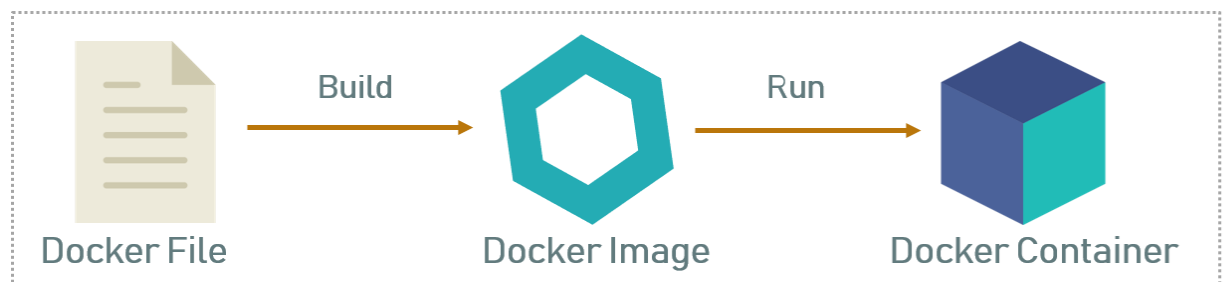
Figure 3. Process of creation of a Docker container from Dockerfile
