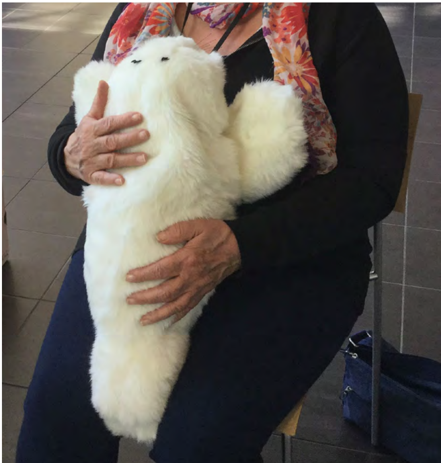
Image 4. The Paro robot seal is a social robot that is used, for example, as a therapy device for people with memory disorders. Image: Toni Pekkola)
