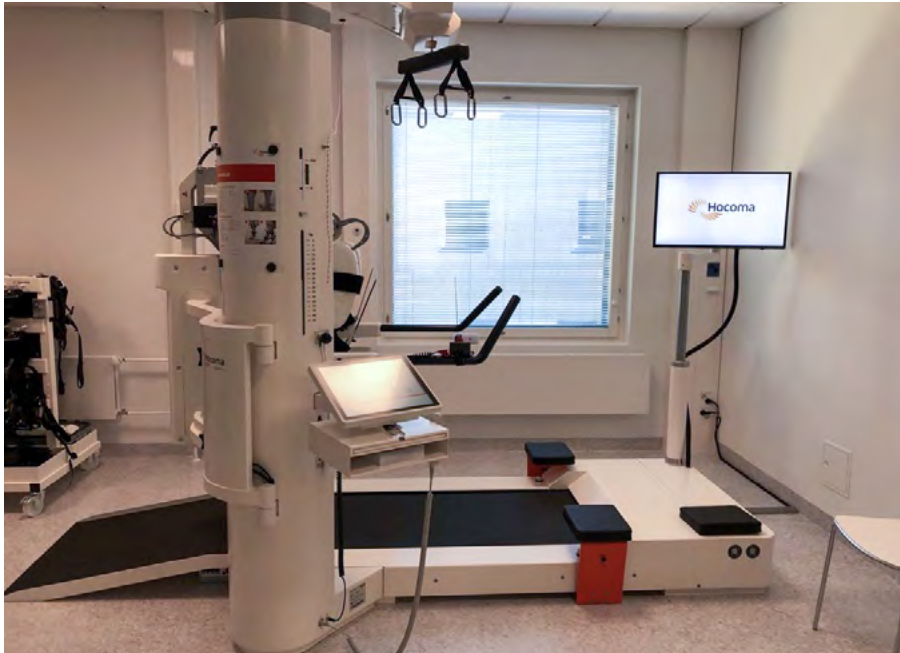
Image 2. The Lokomat robot is used in walking rehabilitation. Image: Essi Heimovaara-Kotonen)
