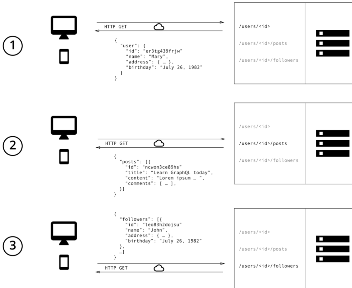
Figur 5. Data Fetching with REST vs GraphQL. (howtographql.com, 2022)
