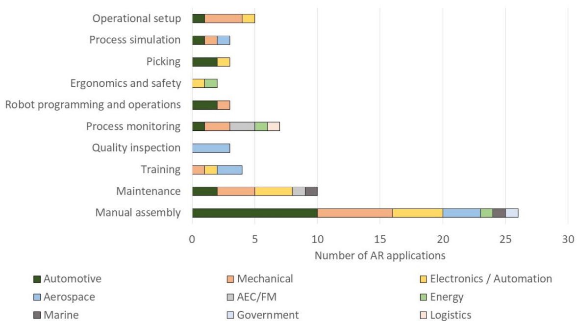
Figure 6. IAR application in different industrial segments (De Souza Cardoso et al., 2020, p. 8)
