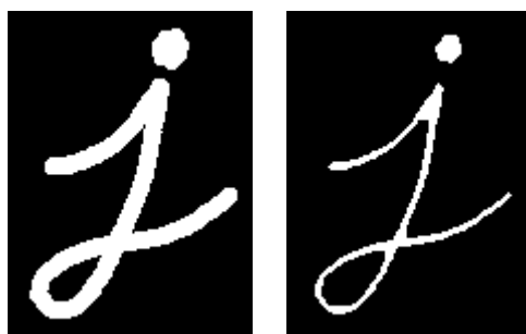
Figure 32 Applying erosion, (OpenCV tutorials 2014.)
