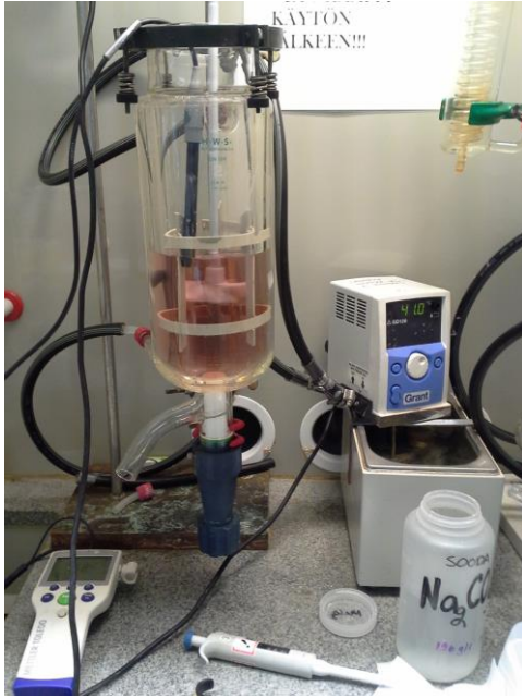
Figure 5. The Reactor and a Water Bath Used in the Experiments
