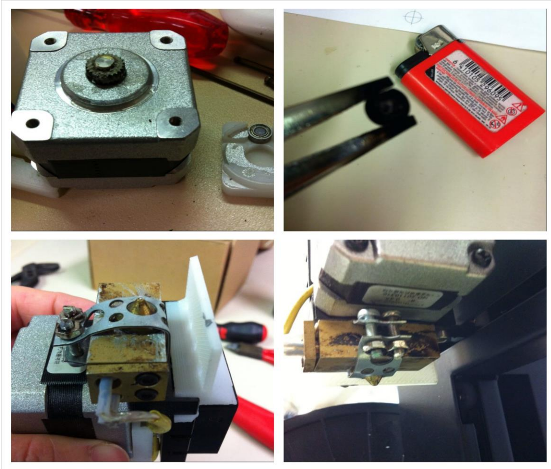
Picture 13: Left up: stepper motor with powder lubricant, Right up: the nozzle heated by lighter, Left down: nozzle fixed by metal ring with screws, Right down: fixed nozzle. From: Lin Zeyu
