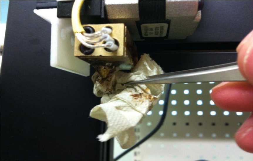
Picture 14: Clean the nozzle with soft paper. From: Lin Zeyu
