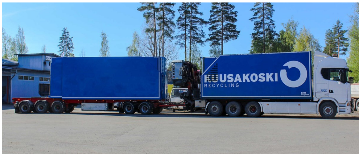
FIGURE 4. Truck-trailer combination suitable for the long-haul transportation of bales and loose silage. Source: (Riiko oy 2022).
