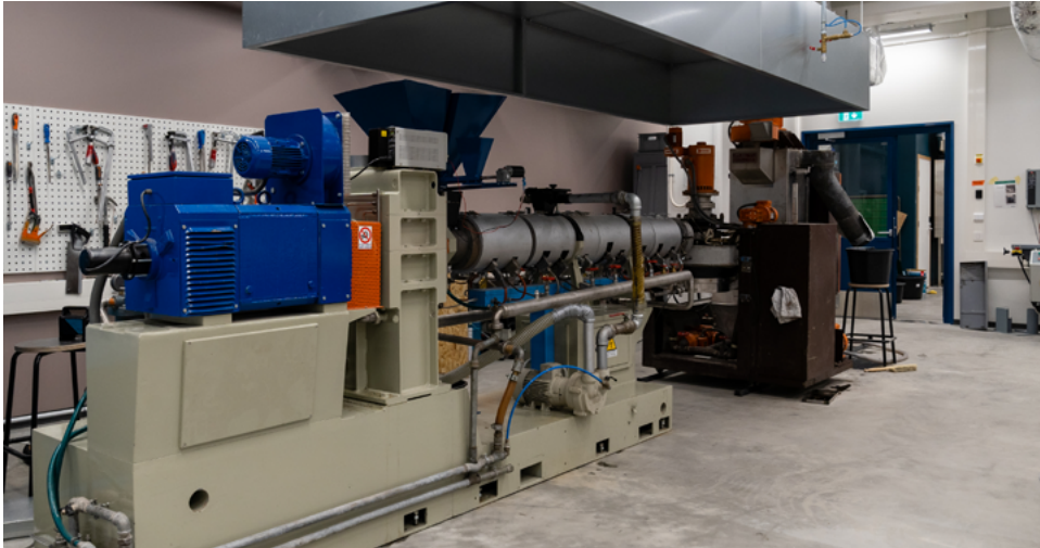
Image 2. The double-screw extruder of the SuMa laboratory (Image: Joni Alhonen)
