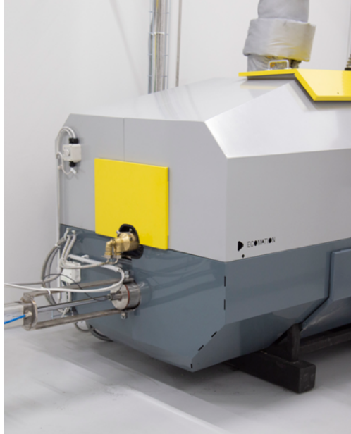
Image 1. Pyrolysis reactor of LAB University of Applied Sciences (Henttonen 2021)
