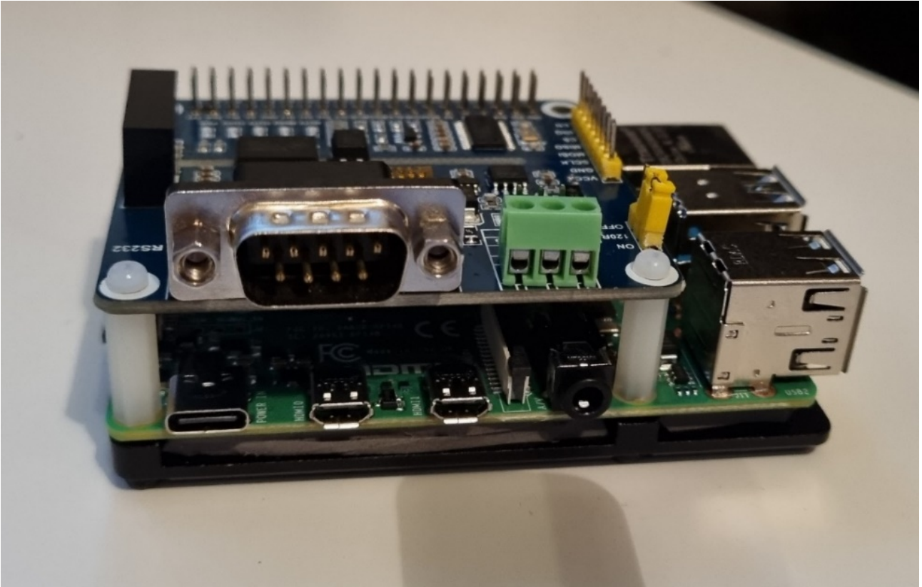
FIGURE 24 RPi 4 with Waveshare Isolated RS485 RS232 HAT installed
