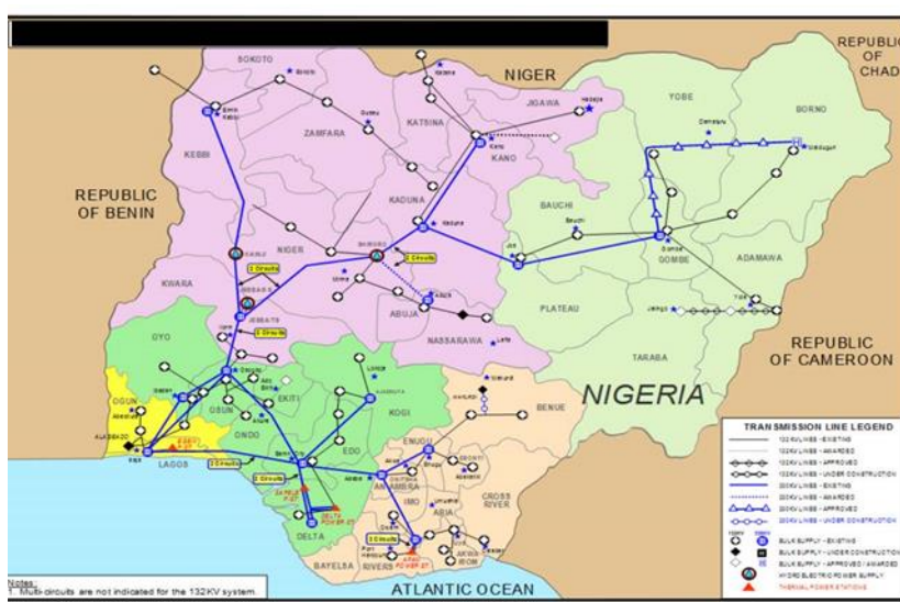
FIGURE 4. Nigeria Transmission Network (NERC, 2021)
