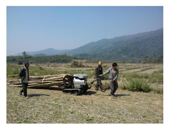
Picture 14. Skidding with the locally manufactured iron horse
