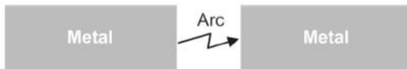
Figure 18: Non-contact arcing due to voltage breakdown
