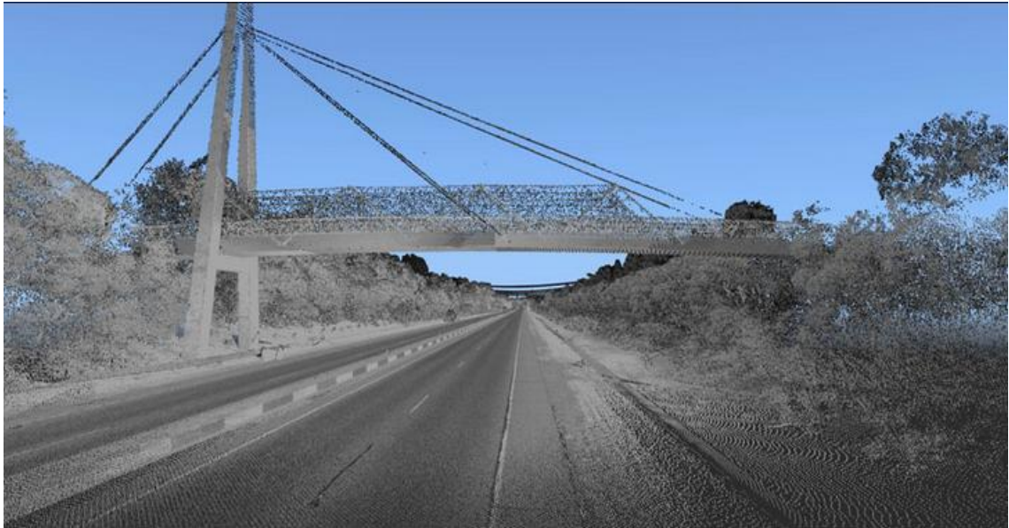
FIGURE 11. Example of a model constructed from point cloud acquired by Mobile Mapper (IGI 2013)
