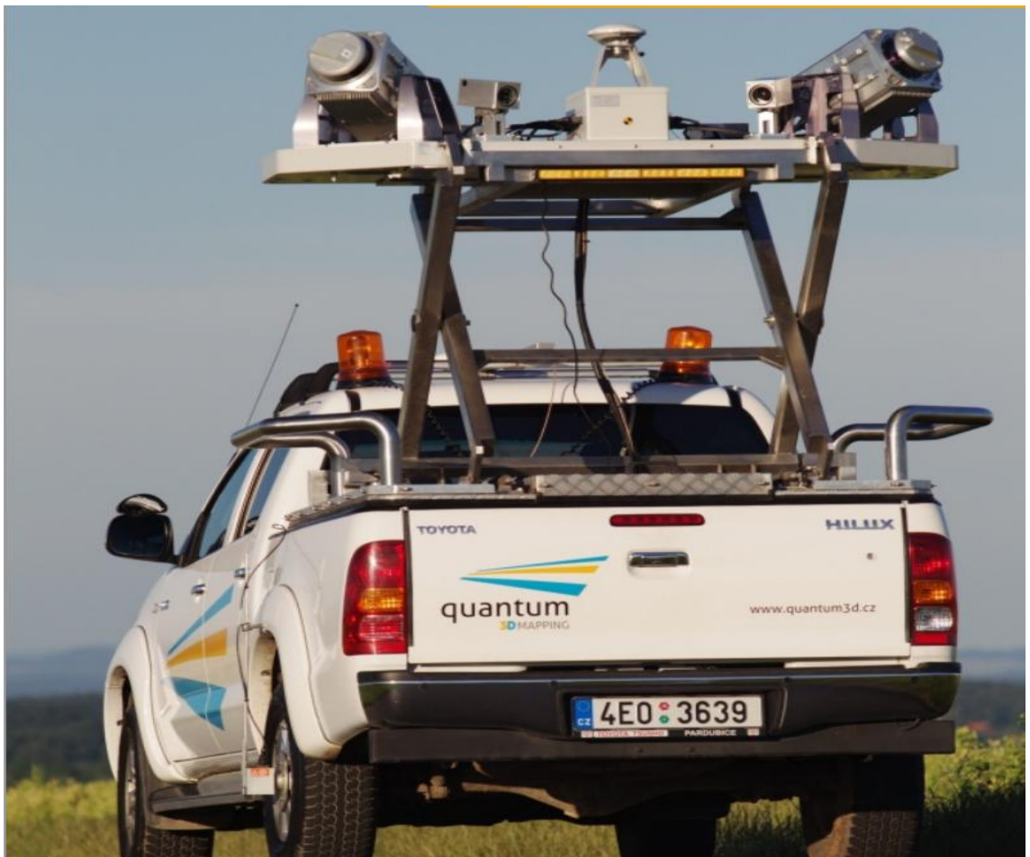
FIGURE 10. Quantum 3D Mapper in operation mode with platform at the height of 3 m (Geovap 2013)
