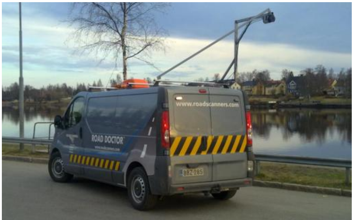
FIGURE 8. Survey van equipped with LMS 151 laser scanner (Matintupa & Saarenketo 2011, 8.)
