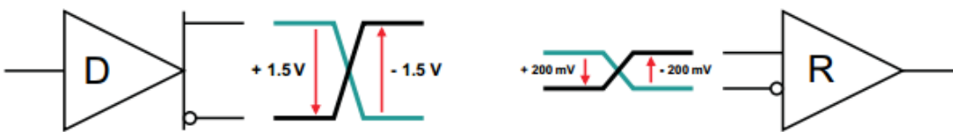
Fig. 10 RS-485 specified minimum signal levels [8 page 2]
