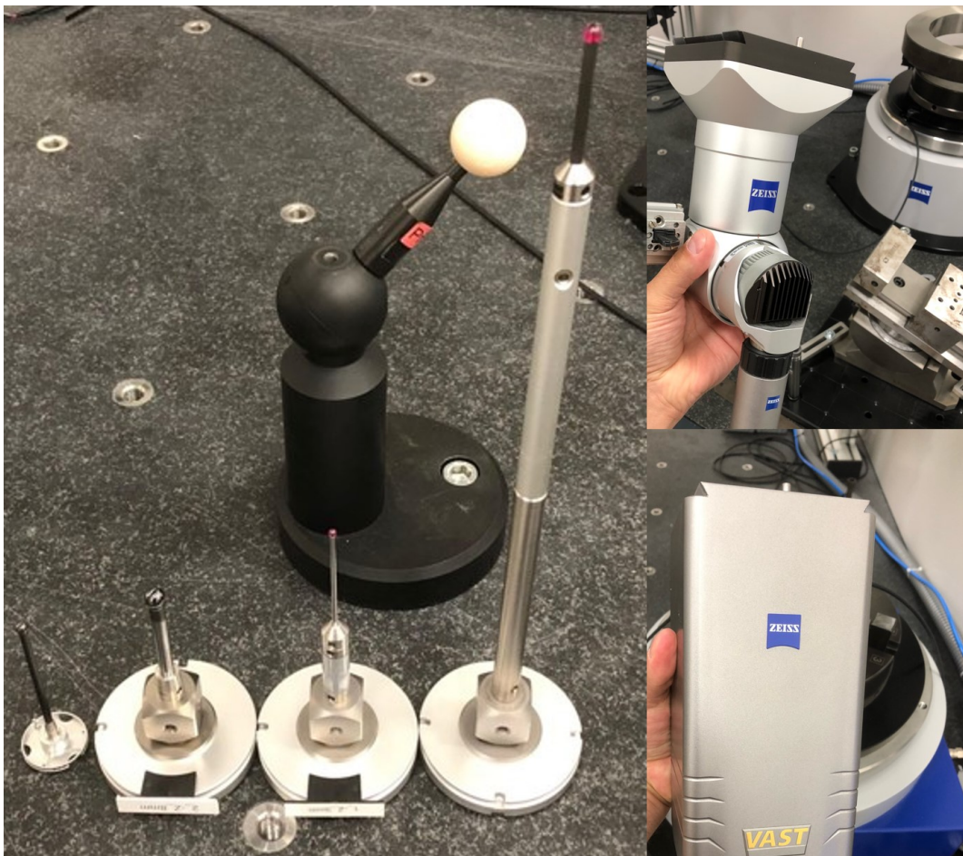
Figure 60. Stylus and sensors for gauge ring measurements.
