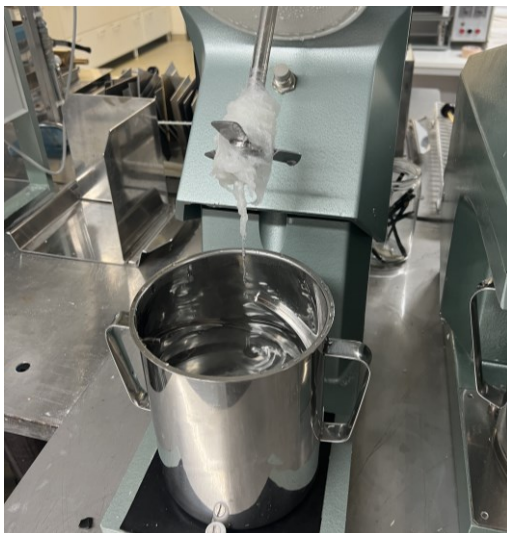
PICTURE 10. Fibres wrapped around the mixing blade.
