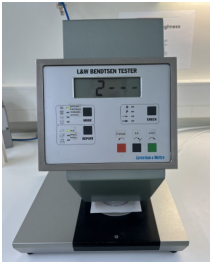
PICTURE 9. L&W Bendtsen Tester.
