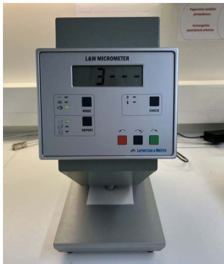
PICTURE 6. L&W Micrometer.
