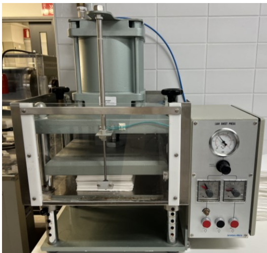
PICTURE 4. Sheet pressing with L&W Sheet Press.
