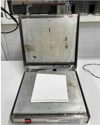
PICTURE 5. Sheet drying with L&W Rapid Dryer.
