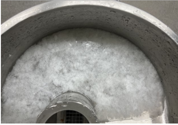
PICTURE 13. Polyester fibres after 10 minutes of refining.
