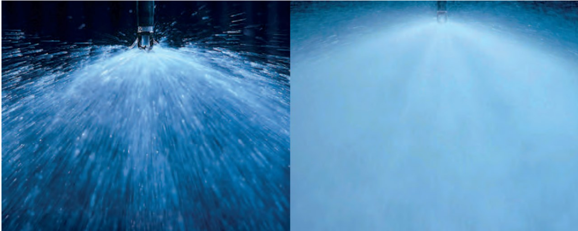
Figure 22. The difference between a sprinkler- and water mist system is in the size of the water droplet. Sprinkler system to the left. (Rakennustietosäätiö RTS, 2012, p. 5)
