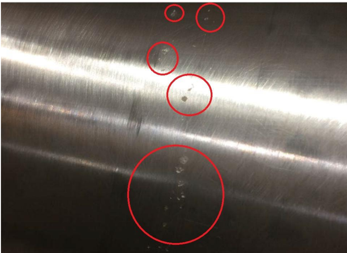
FIGURE 30. Marks on bearing surfaces caused by sparking through the oil film (19)
