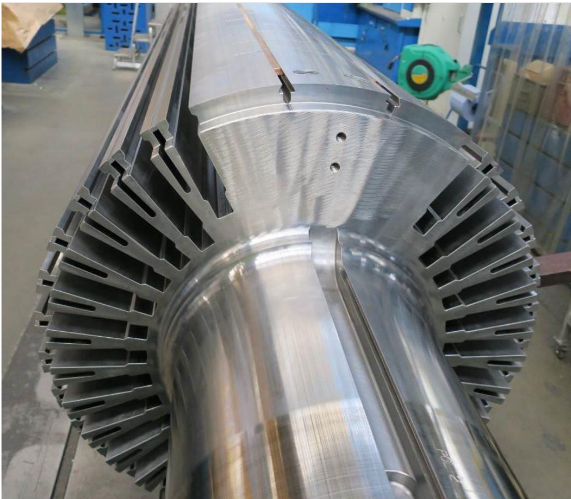
FIGURE 31. Cylindrical pole rotor forging (19)
