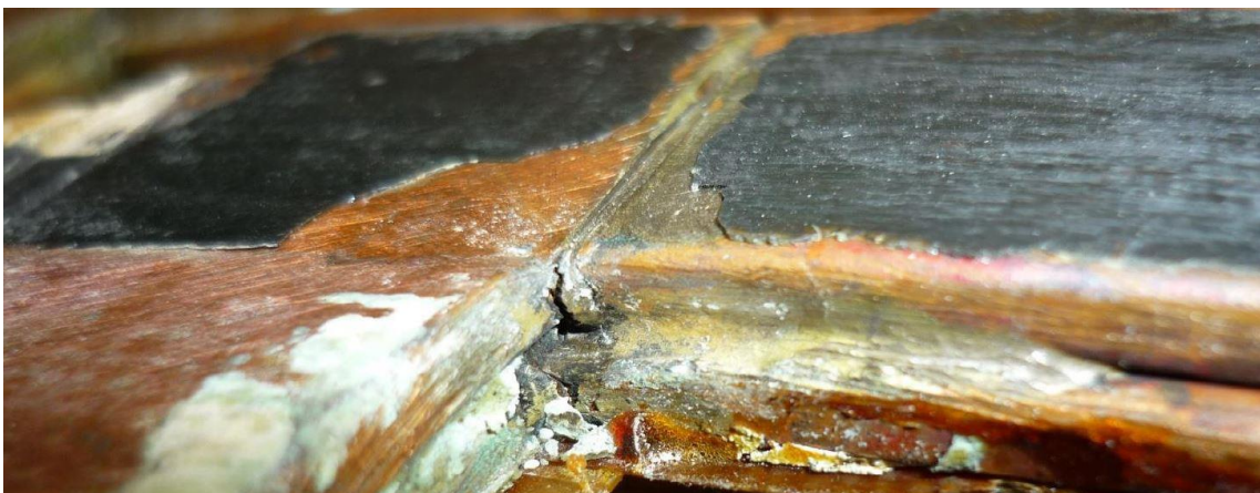
FIGURE 40. Fractures in soldered corner connections (19)
