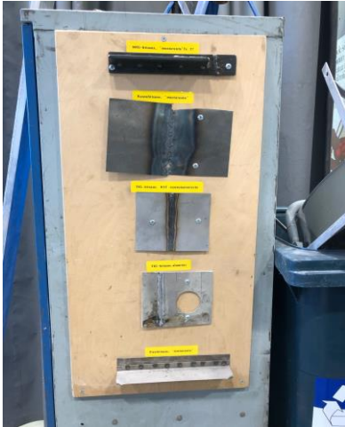
FIGURE 39: a reference guide showing metal plates attached to a plywood sheet made of different material and what welding method is required.
