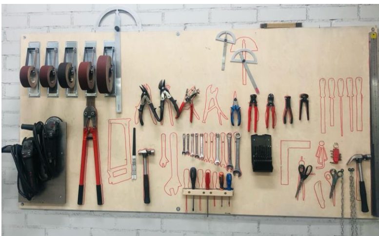
FIGURE 31: Tool wall in Metal workshop in Väre. Outlines clearly indicate which tools are in use or missing. Also notice that some tools are placed in the wrong area.
