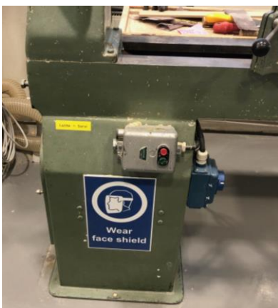
FIGURE 7: Sign reminding to Wear a face shield on the lathe in Construction Workshop. The yellow tape also has the name of the machine in English and Finnish.
