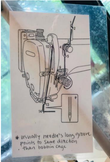
FIGURE 40: Set Design Workshop laminated diagram showing how to setup the thread on the sewing machine.
