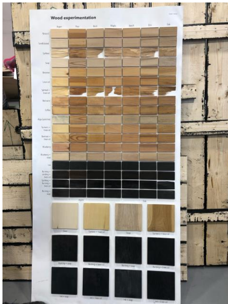
FIGURE 44: A reference chart made from dozens of pieces of wood of varying species oiled or stained with different materials.
