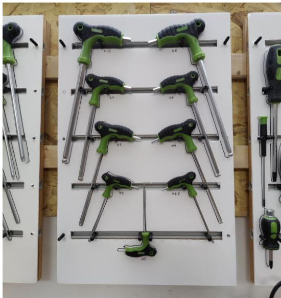
FIGURE 33: A CNC machined wood and aluminium T-slot profiles and mounting with architectural foam board shadows and labelling.
