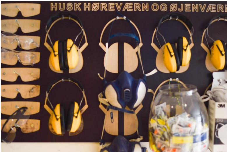
FIGURE 34: CNC cut shadow wall for PPE.
