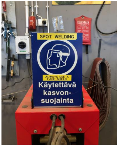
FIGURE 8: Construction Metal Workshop PPE sign. saying always use a face shield when using the Spot Welder in English and Finnish.
