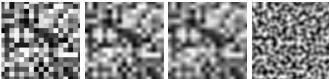
IMAGE 6. The stages of coherent noise generation in 2 dimensions. From left to right: integer-noise, linear interpolation, cubic interpolation and Perlin noise. Image from LibNoise (19).
