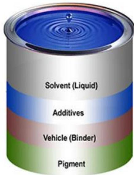
Figure 18: Common components in a coating. (Dean, 2021)
