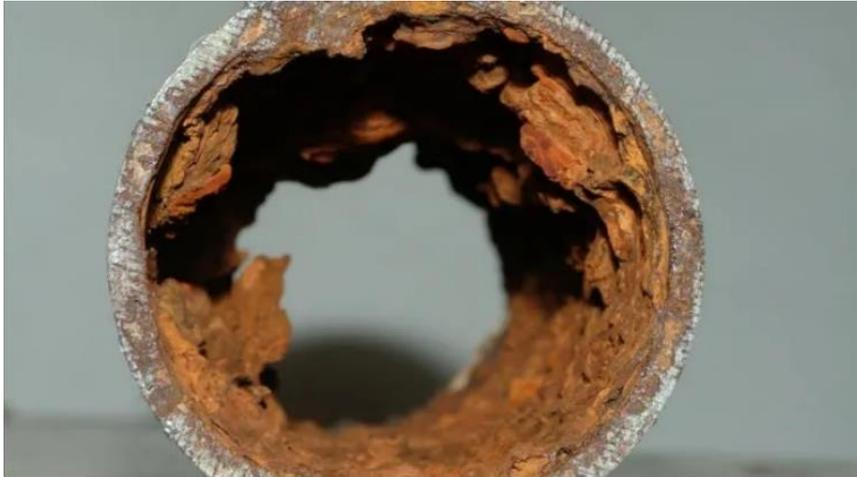
Figure 14: Microbiological Influenced Corrosion (Rope, 2020)
