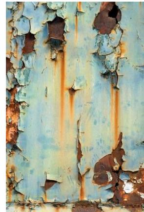
Figure 8: Selective corrosion on shell plate (Moriber, 2020)
