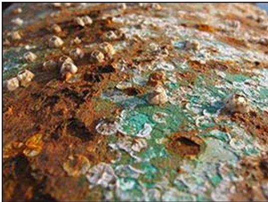
Figure 1: Corrosion (Scherson, 2015)
