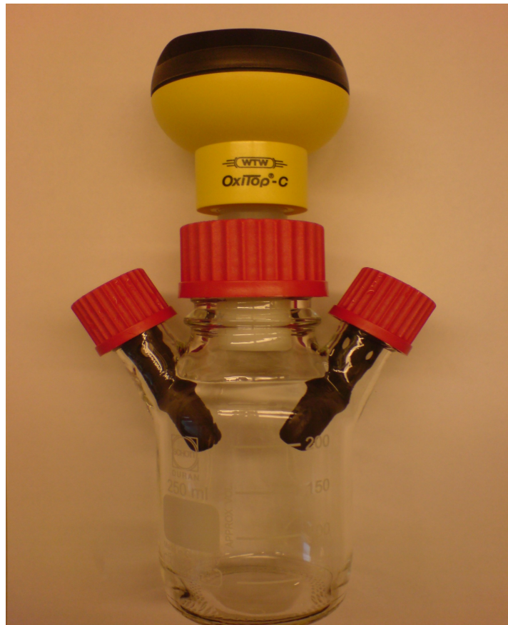
Figure 1. The Oxitop® Sample Bottle with a measuring head
