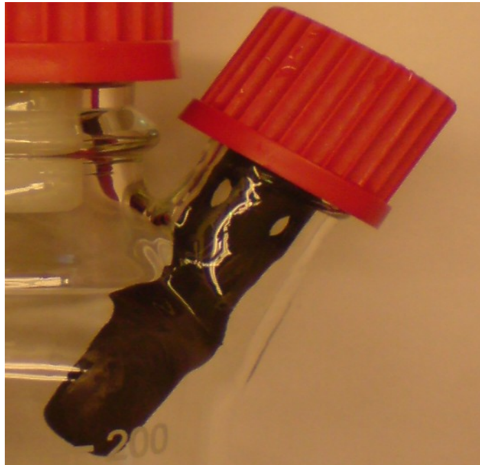
Figure 4. The Septum Nozzle and the Rubber Stopper
