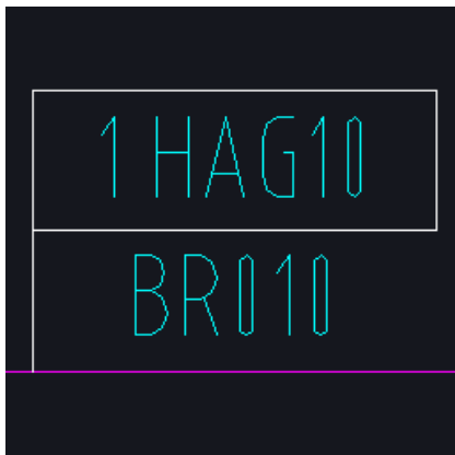
Fig.2 “flag” symbol for pipeline from circulation water pump unit to boiler LP evaporator section. Flow direction from left to right.
