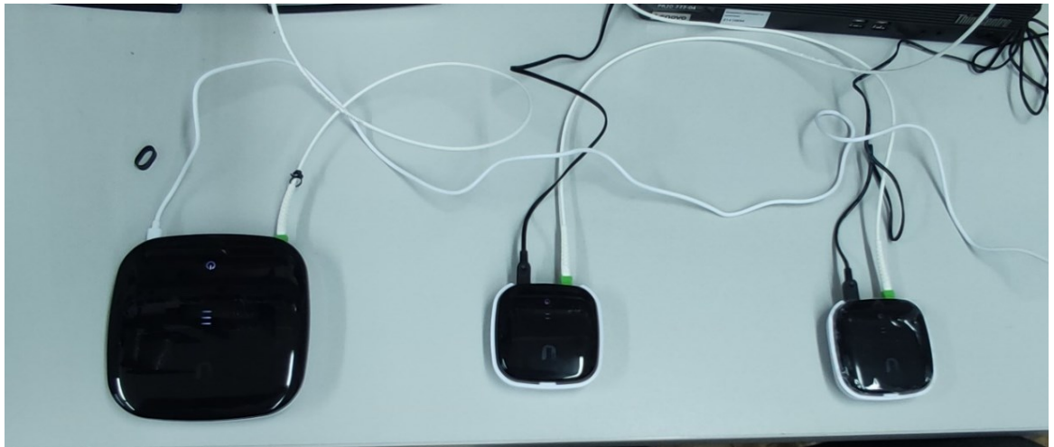
Figure 15 Optical network devices (ONT-left and ONU-right)
