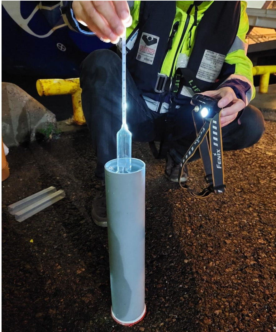
Figure 4 Inserting a hydrometer into the water sample (Forsberg M., 2022)
