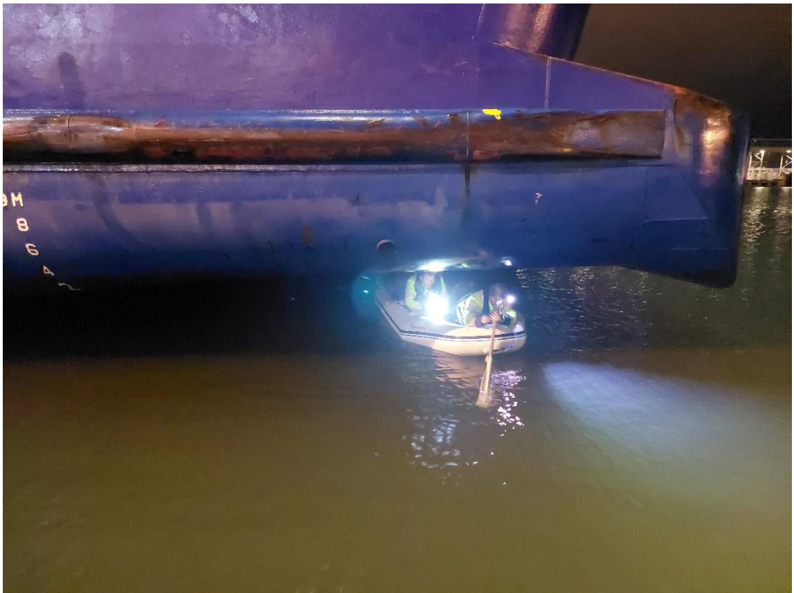
Figure 6 Reading aft draft marks (Forsberg M., 2022)
