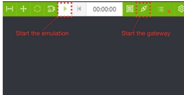
Figure 52. Simumatik's emulation interface
