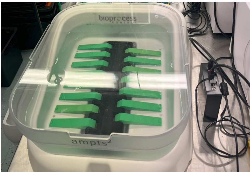
Figure 22. Gas volume measuring unit filled with distilled water.
