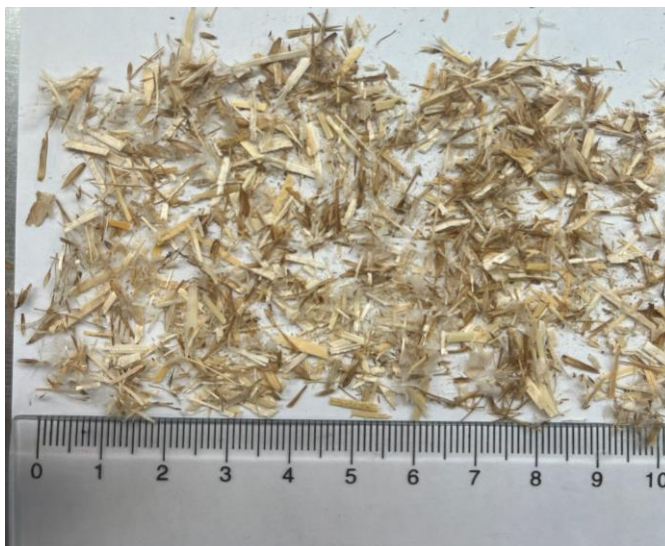
Figure 13. Shredded Winter Reed with a Scale as a Comparison Tool
