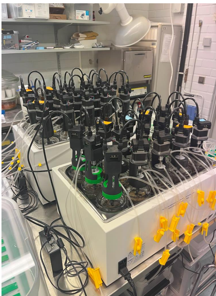
Figure 23. Reactor Setup with Agitator Fully Prepared for Initiation, Complete with All Necessary Tubing and Cable Connection.
