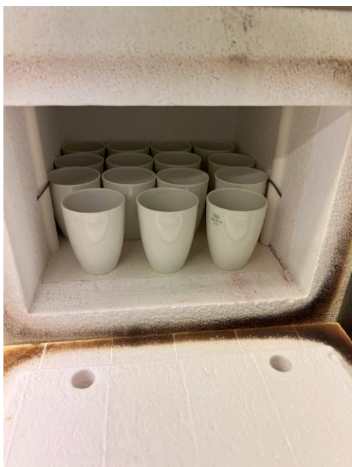
Figure 19. Crucibles Inside the Furnace.
