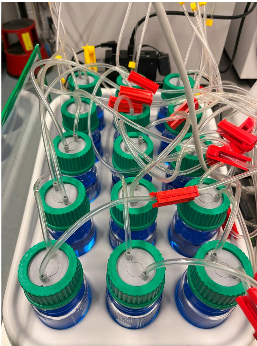
Figure 21. CO 2 -absorbing Unit with Tubing.
