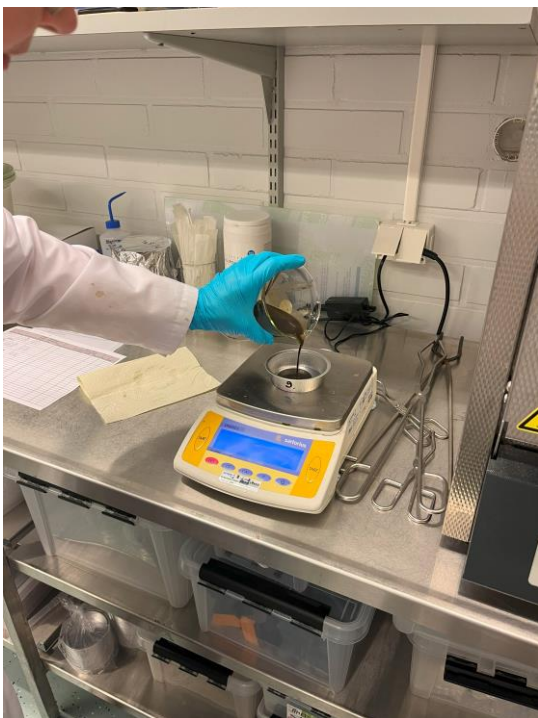
Figure 16. Substrate Weighting Procedure: Adding Substrate to an Aluminum Tray Placed on a Scale
