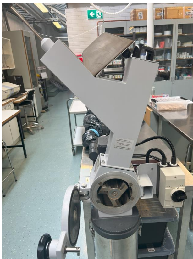
Figure 12. Laboratory Shredding Machine by Retch
