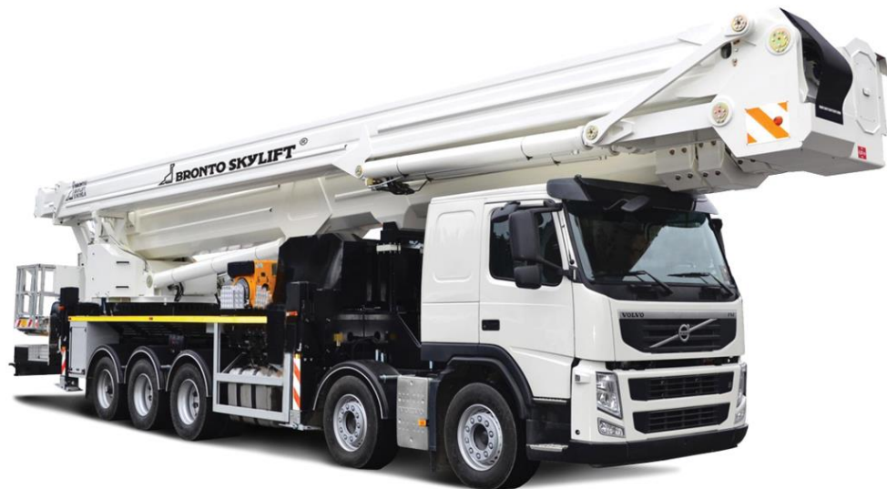
FIGURE 4. Truck Mounted Aerial Platform, Bronto Skylift, S 90 HLA. (Bronto Skylift Website)
