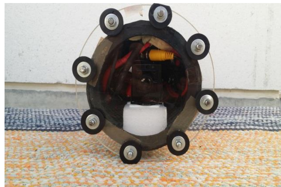
Figure 9. Main tube front view with camera attached.
