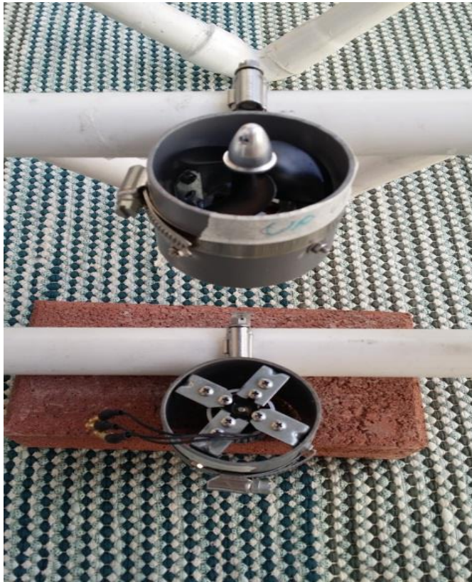
Figure 12. DIY EDF type brushless motors
