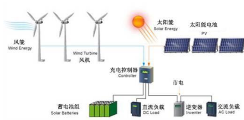
Figure 1: The Component of wind-solar hybrid streetlights (The Wind-Solar Hybrid Power System)
