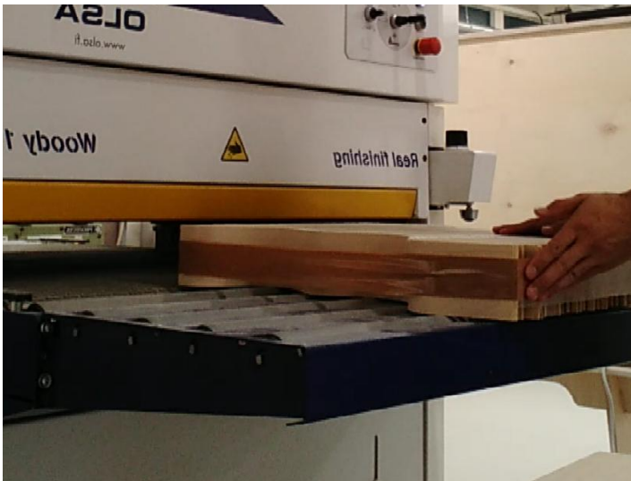
Image 7. Example of an industrial sanding machine
