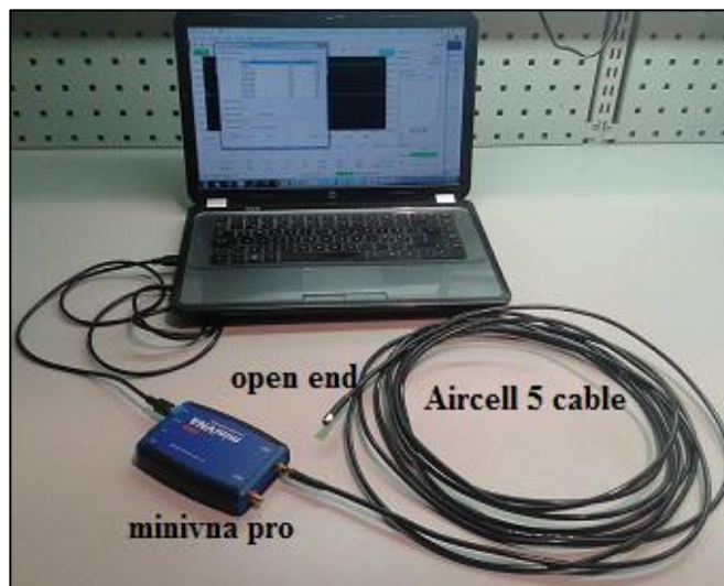
Figure 34: Equipment setup for cable length by using Minivna pro.
