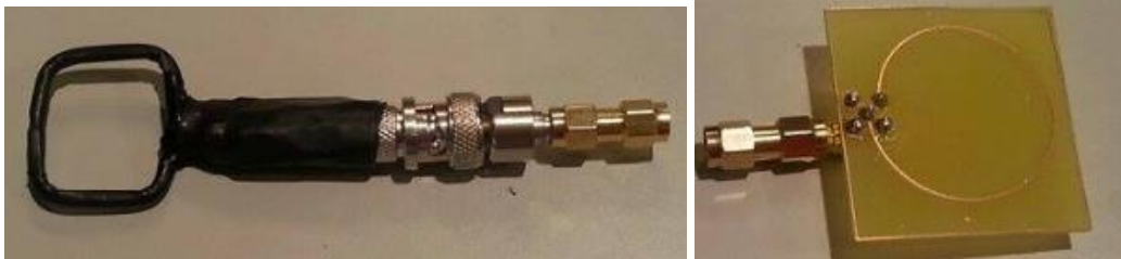
Figure 57: Loop antennas given by supervisor and made in lab respectively.
