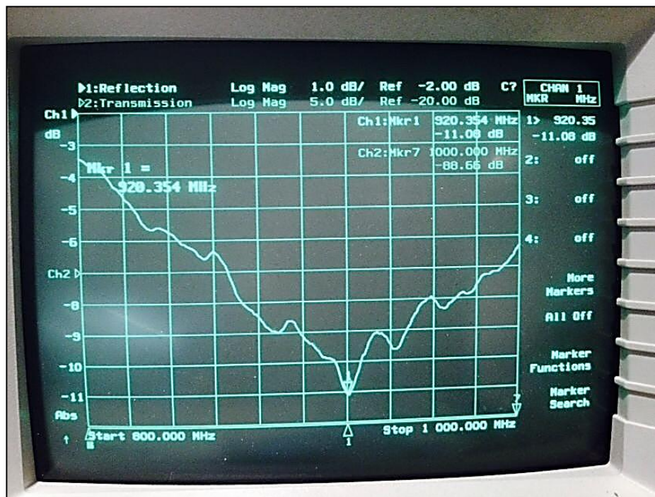
Figure 51: Result after matching monopole antenna from HP VNA.
