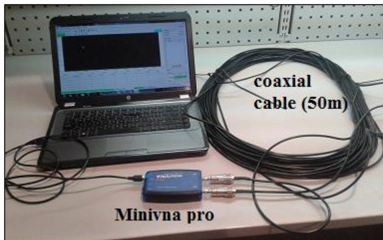
Figure 30: Equipment setup for coaxial cable attenuation by Minivna pro.
