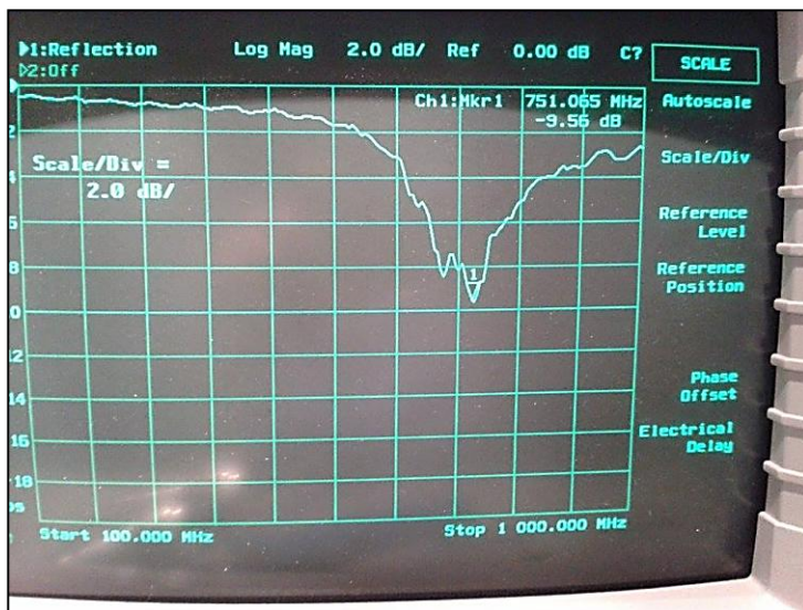
Figure 55: Result for monopole antenna of 10cm length from HP VNA (751.065MHz).
