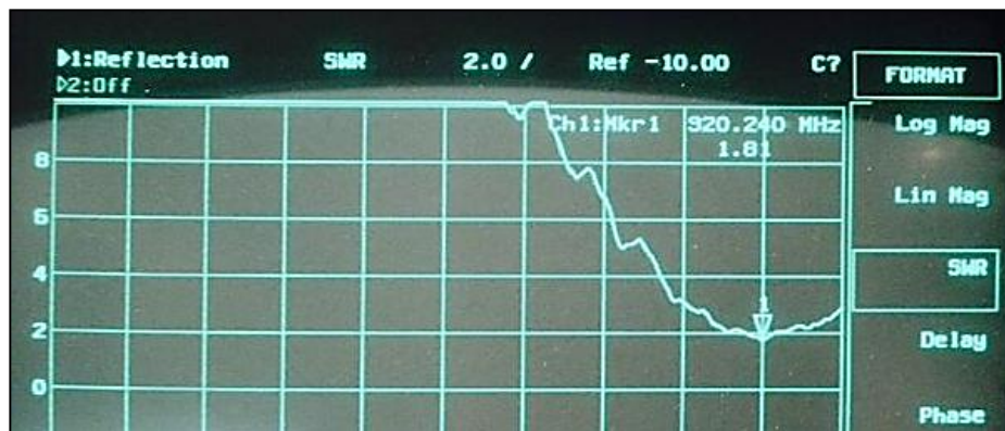
Figure 53: SWR for monopole antenna from HP VNA.
