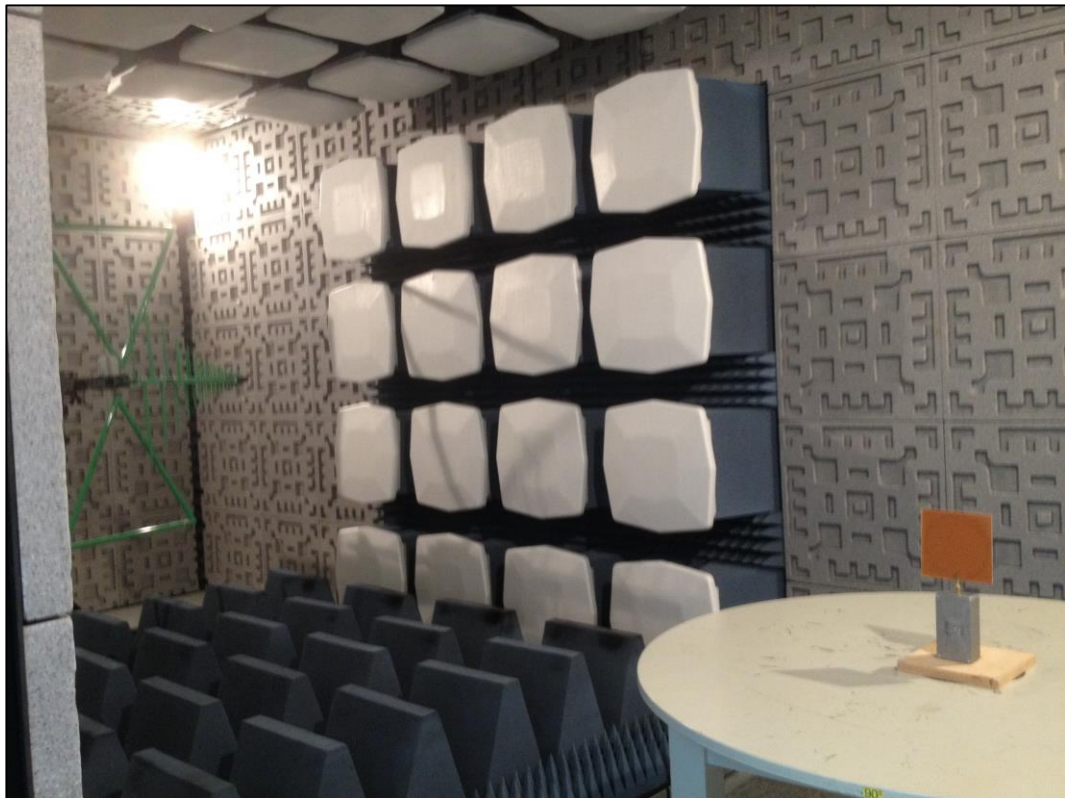
Figure 17. PCB connected to EMI source inside anechoic chamber
