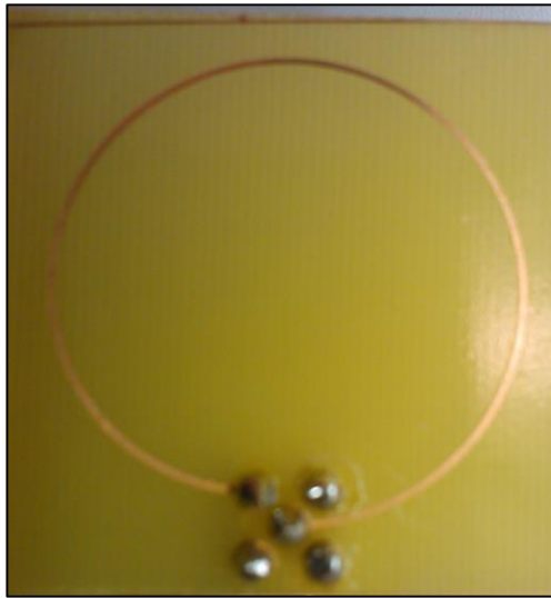
Figure 25. Self-made PCB (small loop antenna without ground plane)
