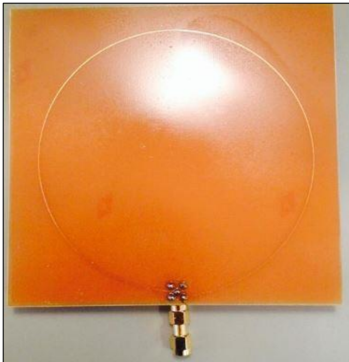
Figure 16. Self-made PCB (closed loop antenna with ground plane)
