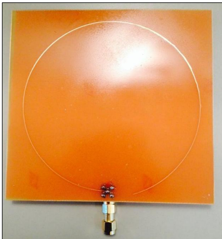
Figure 19. Self-made PCB (open loop antenna with ground plane)
